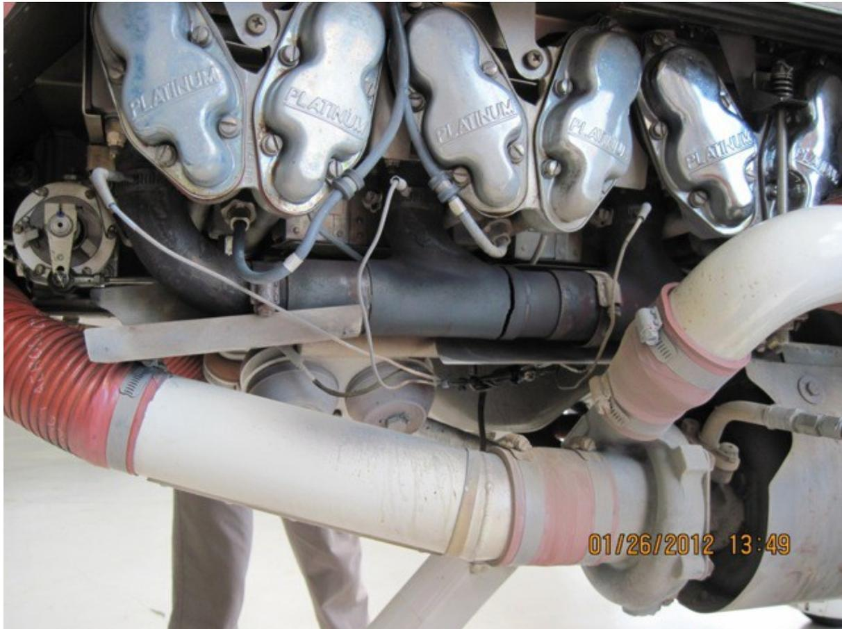
**Continental IO550N Cracked Exhaust Manifold (2), ATA 7810**
